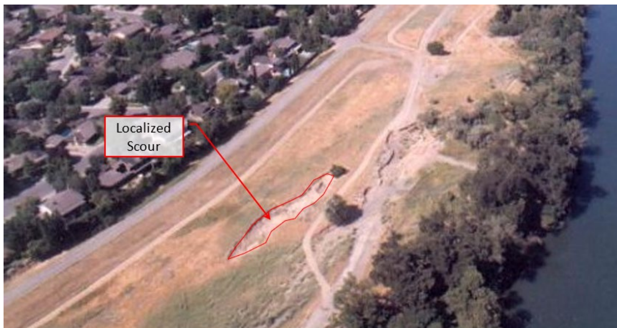
Figure 1. 1986 Flood Event Aftermath On The Lower American River and Localized Lone Tree Scour
