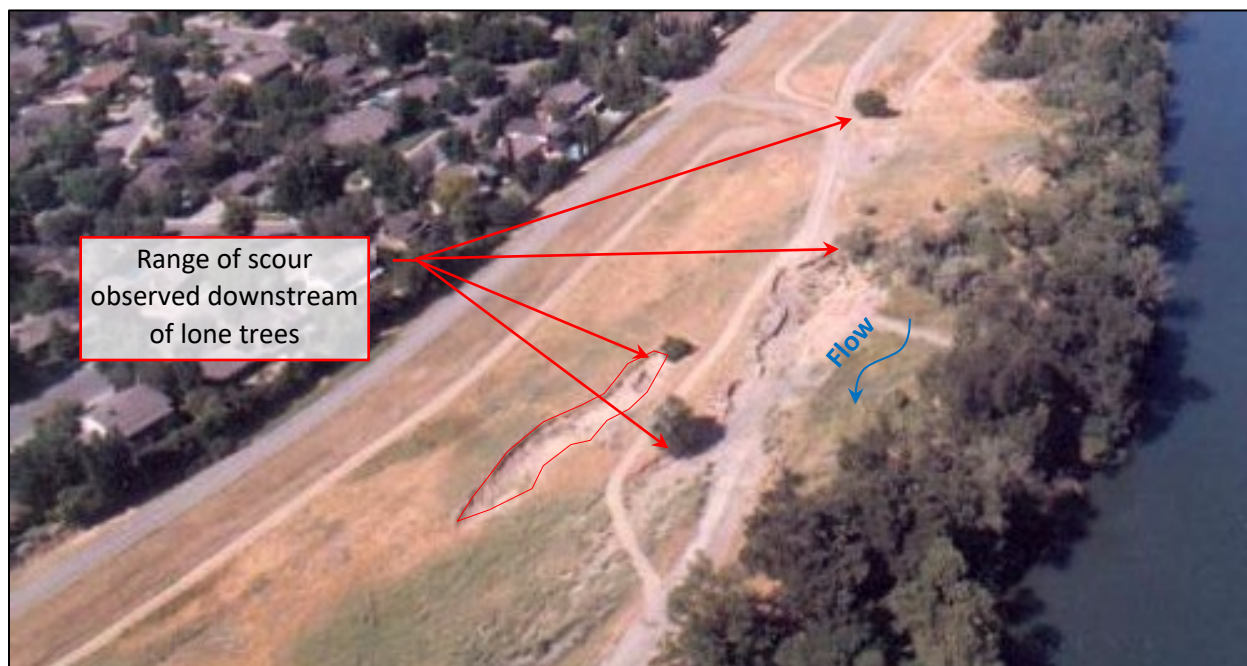
Figure 2-35. 1986 Lower American River flood event aftermath - localized lone tree scour
